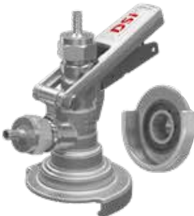
"A" type coupler in st. steel with 5/8" - 5/8" Shank 5235PIA5858.DSR without connections 5235PIA5858.DSI with 7mm nipple, nut and seal 5235PIA3838.DJG with 3/8" quick fitting
