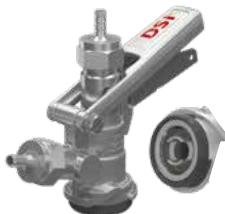
"D" type coupler in st. steel with 5/8" - 5/8" Shank 5235SVD5858.DSR without connections 5235SVD5858.DSI with 7mm nipple, nut and seal 5235SVD5858.DJG with 3/8" quick fitting
